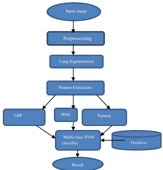
Fig.5 System Architecture.
