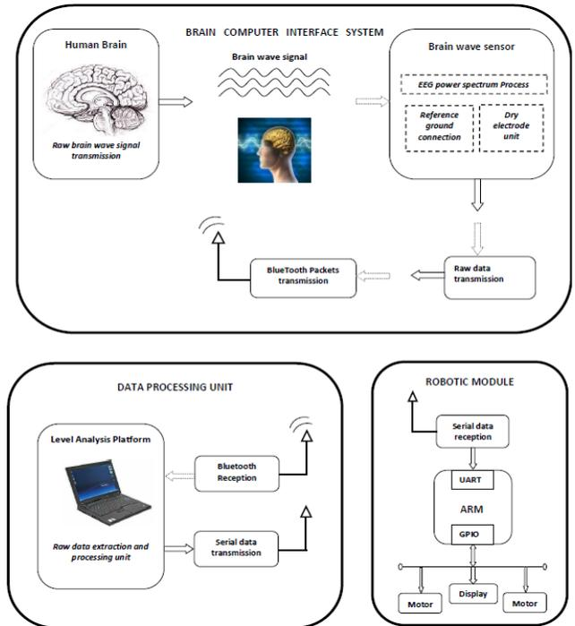
Fig.1 Block Diagram of brain computer interface system.
