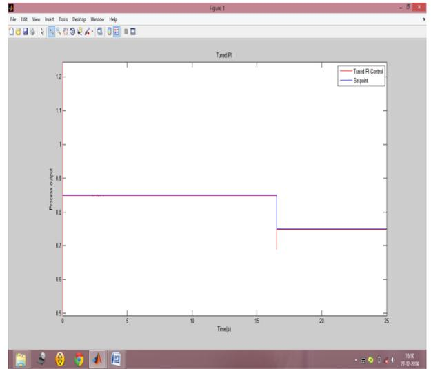
Fig.5 Dynamic set point tracking using tuned PI Controller
