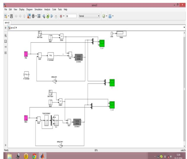
Fig.3 Simulink model for fault tolerant DC motor speed control
