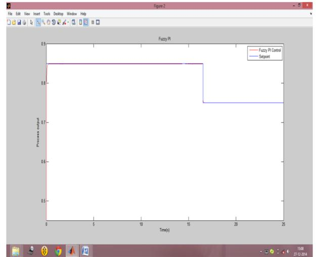
Fig.6 Dynamic set point tracking using fuzzy PI Controller
