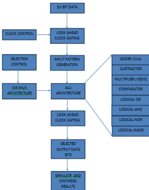
Figure 1. Block Diagram of ALU Architecture
