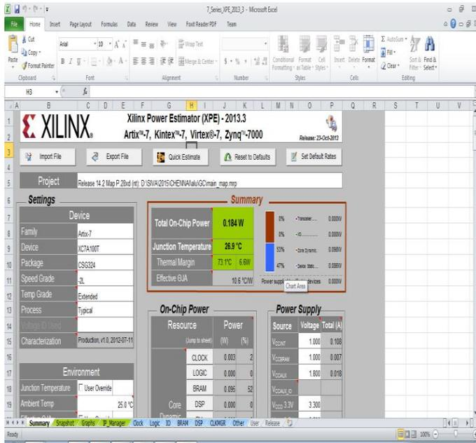
Figure 7. Power Analysis of 32 Bit ALU Using Look Ahead Clock Gating Technique
