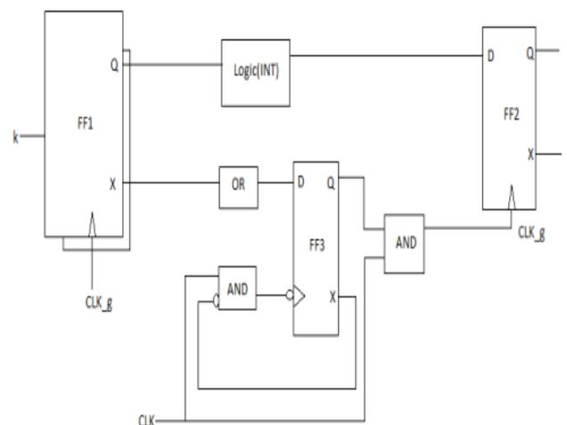
Figure 2. Block Diagram Look Ahead Clock Gating
