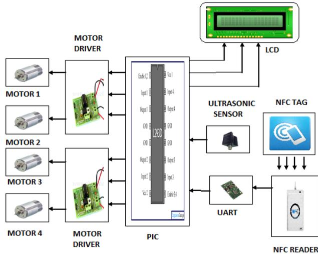
Fig.1 Basic Architecture of NFC Reader
