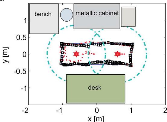
Fig.2 Cell partition in the case of three tags
