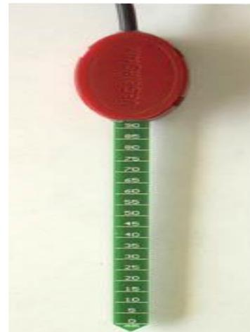
Figure.3 Soil Moisture Sensor
