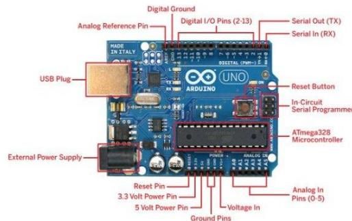
**Fig 2: Arduino Uno Microcontroller**
