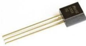
**Fig 3: Temperature Sensor**
